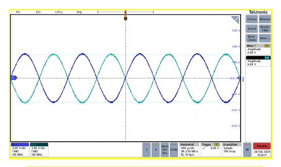
Measured output of ifi Zen DAC V2 left channel balanced outputs with respect to ground.
